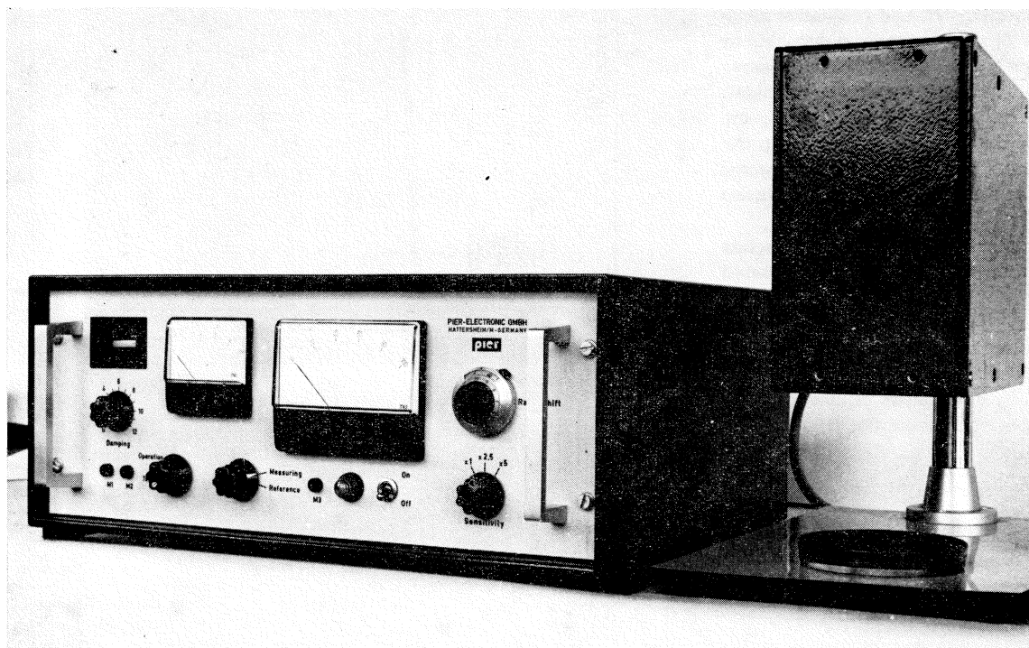
Fig. 2. — Pier electronic moisture meter
