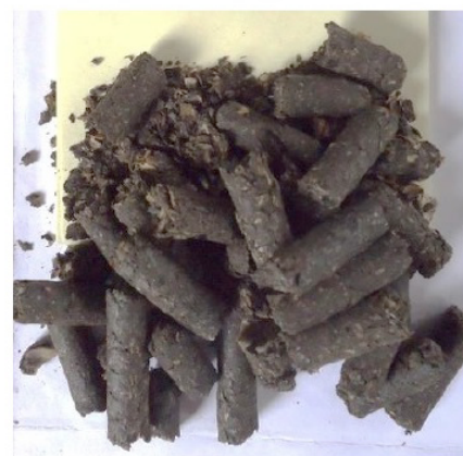
Figura 2.3.2. Pellets from 70% pulp coffee and 30% husk coffee
