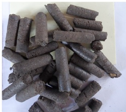
Figura 2.3.1. Pellets from 100% pulp coffee
