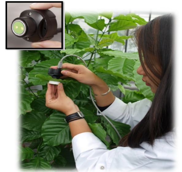
NIR Hand-held Analyzer taking readings in coffee leaves
