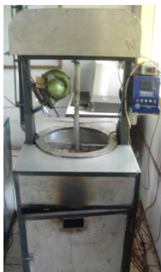
Figure 1. Pilot scale crystallizer designed by ICCRI.
