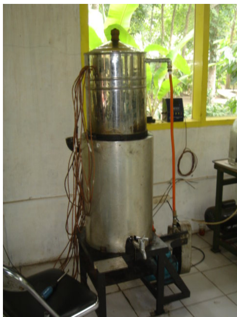
Figure 1. Single column reactor for extraction of coffee powder designed by ICCRI.
