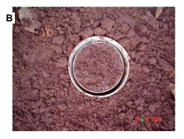
Figure 1. Lysimeter (A) and microlysimeter (B).
