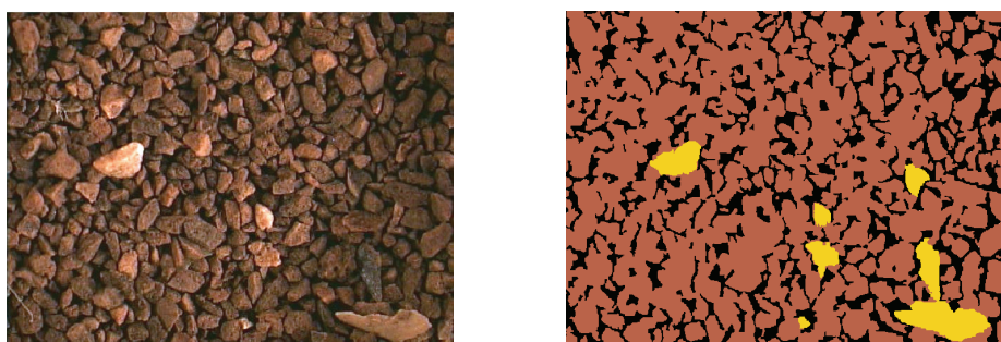
Figure 3. Image of sample processed with 1,5% of impurity.
