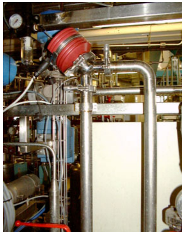
Figure 9. On-line monitoring of total solids using K-Patents refractometer.
