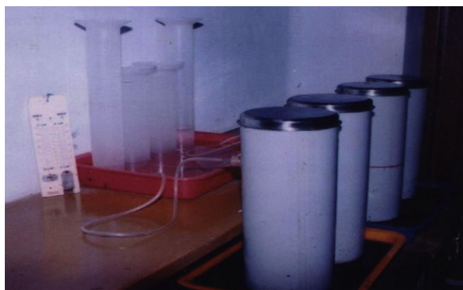
Figure 1. Lab scale fermenter used for biogas production.
