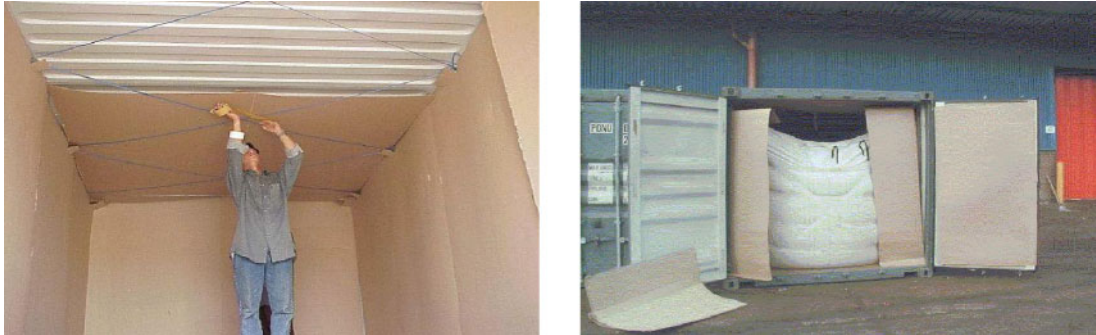
Figure 3. Installation of cardboard and liner.
