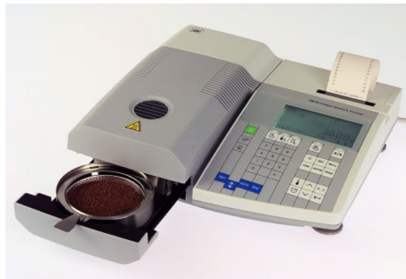
Figure 10. Near-line monitoring of moisture in soluble coffee using a halogen analyser.
