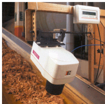
Figure 11. On-line monitoring of moisture in powdered products using NDC MM710. Sensory evaluation
