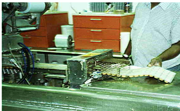
Figure 5. A form-fill-seal machine preparing diet packs; one machine could supply the needs for a whole country's parasitoid production
