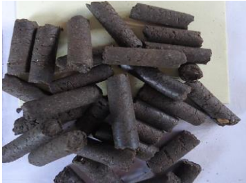
Figure 1: 8 mm pellets from 100% coffee pulp
